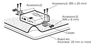
Installation using the self-tapping screws
